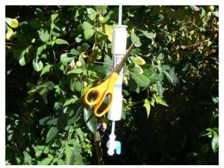
This photo shows that the magnets in the processor are strong enough to hold up a pair of scissors. The ¼ inch tubing is small
